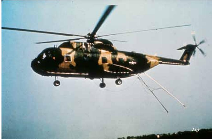
**CH-3 helicopter equipped with the Mid-Air Retrieval System (MARS).**
