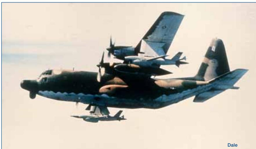
DC-130 drone director aircraft with drones on outboard pylons.
